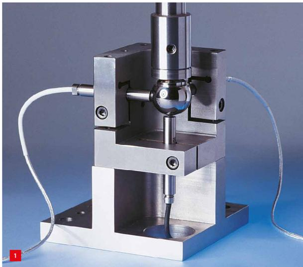
Set-up of a classic thermal distortion test using three capacitance sensors.
