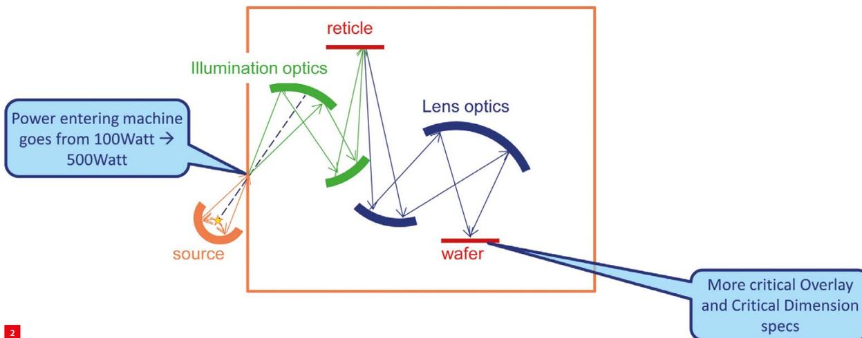
2 Thermal challenges in ASML's new EUV lithography machines.
